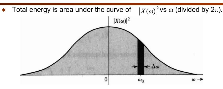
• The energy over a small frequency band  $\Delta \omega$  ( $\Delta \omega \rightarrow 0$ ) is:
